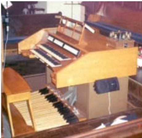
A new console was constructed of ash, with a base which is covered in Formica. Ted remarks that this cured the constant scuffing of the case by people seated in choir pews directly behind the console. The Carter keyboards
