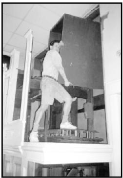
The Swell division is expressive with only two options –open or closed. The horizontal shades close by gravity. The trace is connected to a pedal having a latch (hitchdown) to secure the "open" position.
